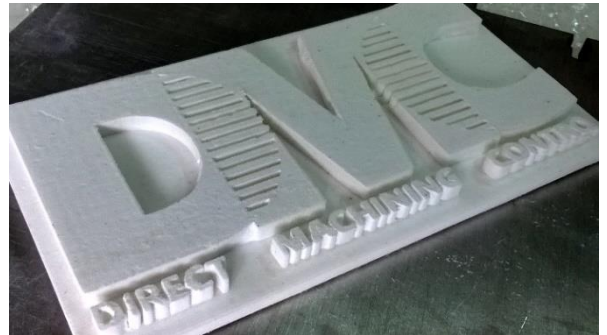
Figure 2 A sample printed via process controller by the DMC software
